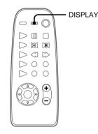
➡ Press DISPLAY when the power is off. The unit switches to the Power Saving Mode and the clock display disappears. The system turns on/off by pressing I/<sup>(1)</sup>.
